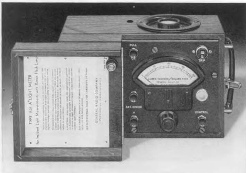
Figure 1. Panel view of the Light Meter, showing meter scale and controls.
