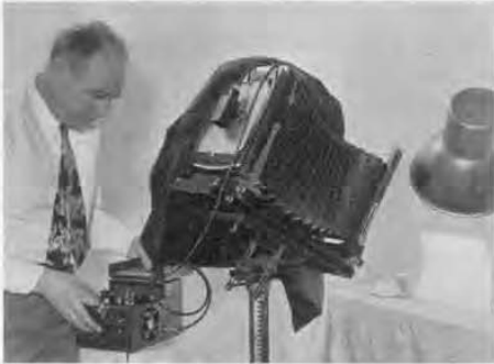
Figure 5. Illustrating use of Type 1501-P1 Probe to measure light reading film. Probe attaches to ground glass with two rubber suction cups.
