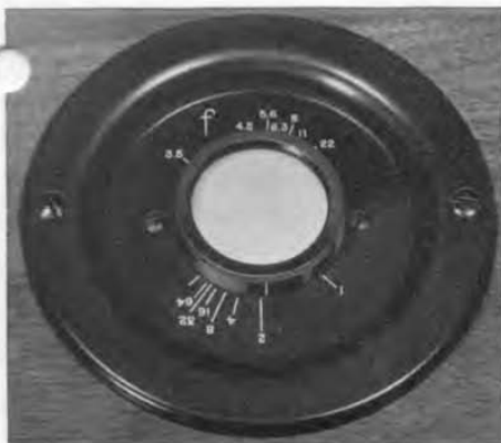
Figure 3. View of the light attenuator, showing f/scale and proportional scale.
